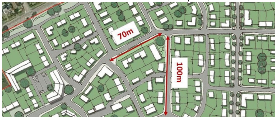
Example of a layout with organic. It is well connected with block lengths between 50m & 100m creating a walkable, permeable layout.
