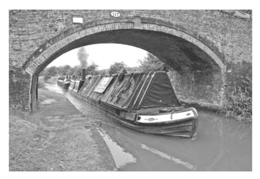
Fellows Morton Clayton narrow boat "Gifford" in tow. The 'President' has a distinctive 'Josher' shaped hull, which has riveted wrought iron sides and a 3" elm bottom. It also has a unique funnel which can be folded when it negotiates tunnels. The specially developed steam engine and coke fired boiler took up so much space in the hull that
